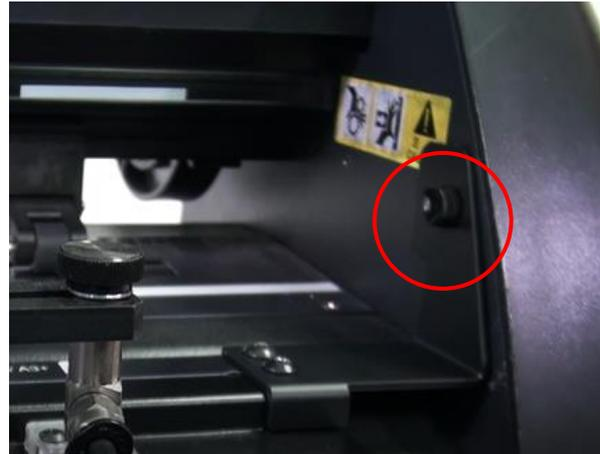
3. Loose the screws on the side brackets of auto feeder.
