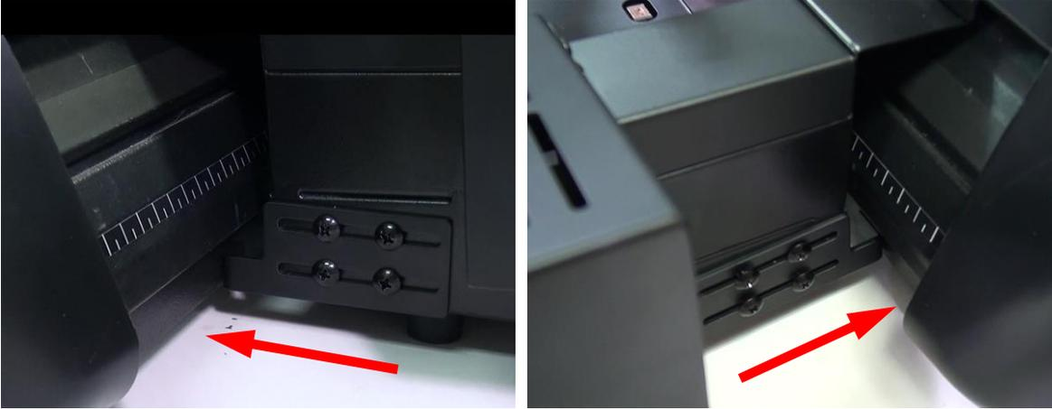
5. Loose the screw on the rear platen.
