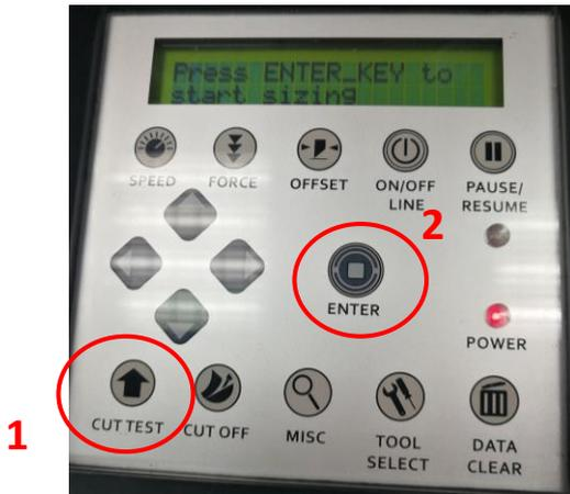
The default cutting force and offset value of the cutting test are 80gf and 0.275mm respectively. Press [ARROW KEY] to move the tool carriage to the position where you like. Then, press the [ENTER KEY] to perform Cut Test.
