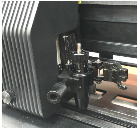
**Step 2** Fasten the thumb screw to fix the tool carriage.
