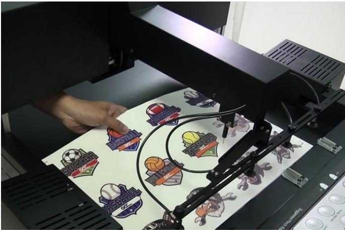
**Step 2** Put the L-type media blocks to touch the rear edge of the sheet media.
