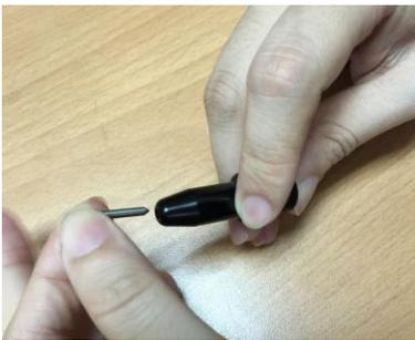
**Step 2** Push the blade to the bottom of the blade holder.
