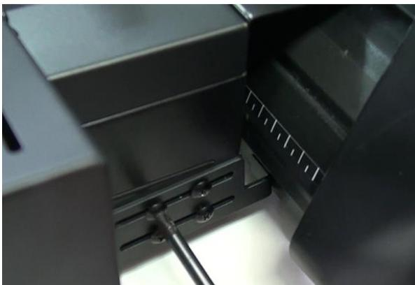
4. Push the side brackets to closely lean against the cutter, and then tighten up the screws.
