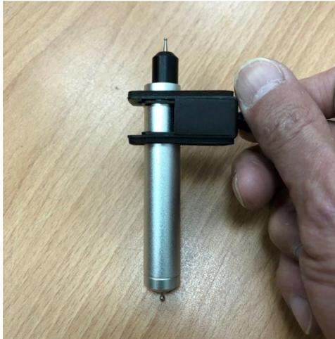
Make sure the tool is insert to the bottom of the holder tube and turn the hand screw to lock its position
