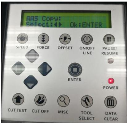
**Step 11** Then use arrow up/down keys to define the repeated value (value = 0- 500) and press “ENTER” key.
