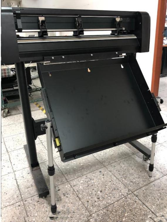
Note: Drawer-type autofeeder design allows users to extend the feeder to accommodate B2 size paper.
